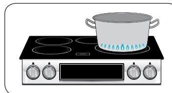
Virtual flame technology creates the appearance of flames when you turn on an induction element.
